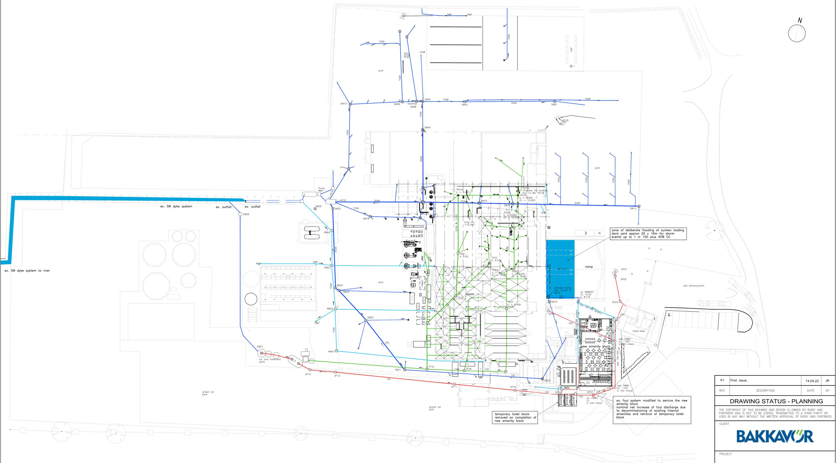
zone of deliberate flooding of sunken loading dock yard approx 29 x 16m for storm events up to 1 in 100 plus 40% CC
