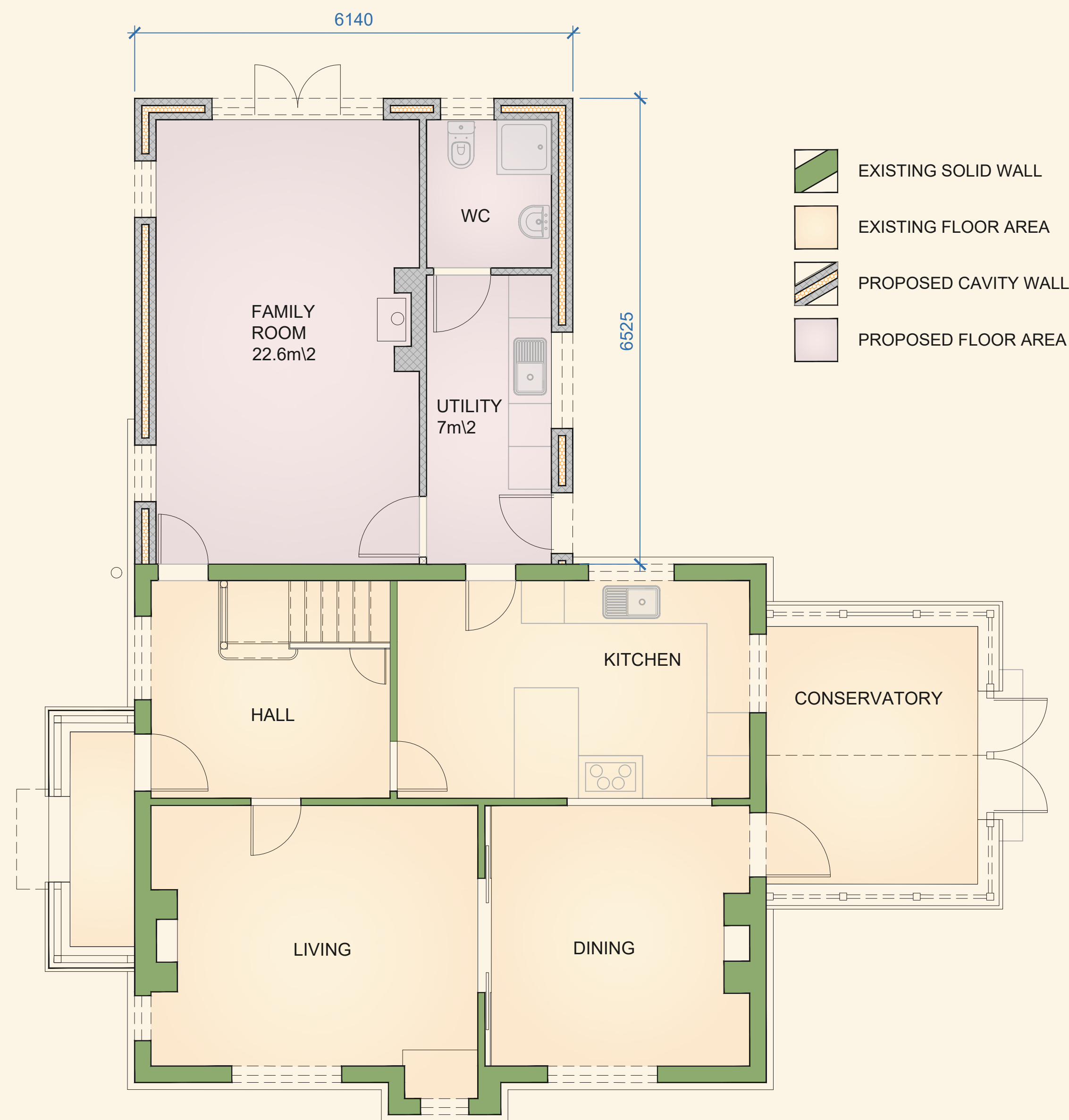
PROPOSED GROUND FLOOR PLAN 1:50
