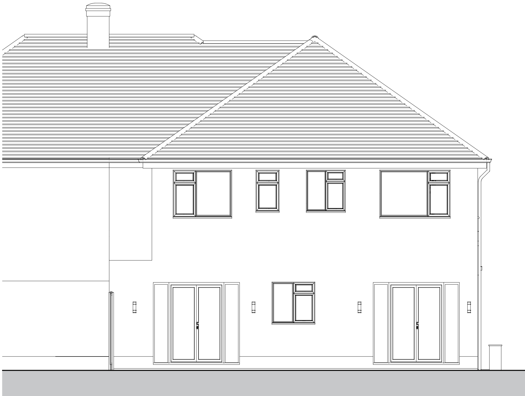
PROPOSED REAR ELEVATION 1 : 50
