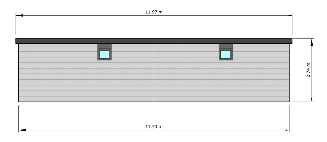
Roof Covering: EPDM seamless roof covering with 10mm gravel top coat. Wall cladding: Composite Shiplap Fascia & soffit: PVCu Anthracite grey Windows & doors: PVCu Anthracite grey 0m
