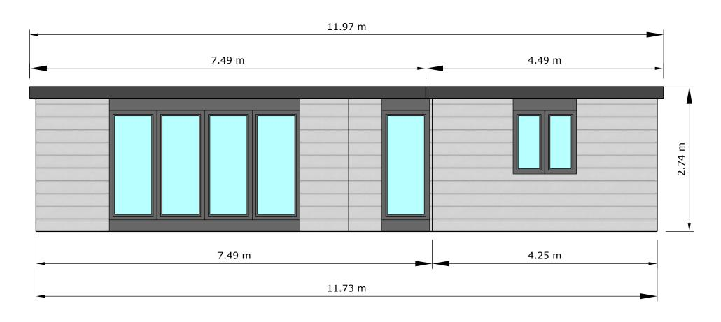
Roof Covering: EPDM seamless roof covering with 10mm gravel top coat. Wall cladding: Composite Shiplap Fascia & soffit: PVCu Anthracite grey Windows & doors: PVCu Anthracite grey
