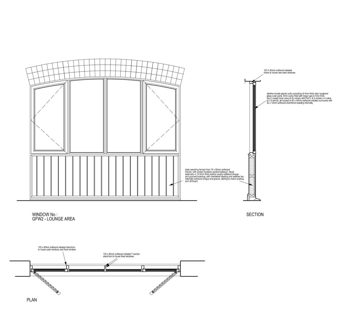
120 x 44mm softwood rebated head and stiles with 20 x 12mm softwood chamfered beading internally to house slimline
