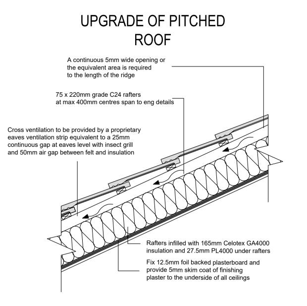
Ensure insulation is installed tightly between the rafters and over rafters to prevent thermal bridging
