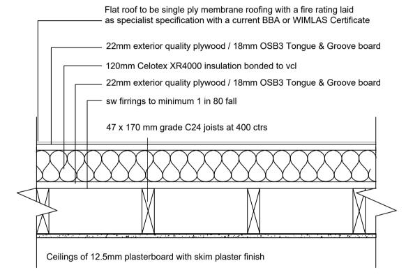
WARM FLAT ROOF (imposed load max 1.0 kN/m<sup>2</sup> - dead load max 0.75 kN/m<sup>2</sup>)
