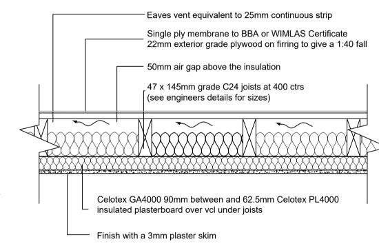
VENTILATED FLAT ROOF (imposed load max 1.0 kN/m<sup>2</sup> - dead load max 0.75 kN/m<sup>2</sup>)
