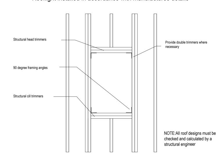
**ROOF LIGHTS** Min U-value of 1.6 W/m<sup>2</sup>K. Roof-lights to be double glazed with 16mm argon gap and soft low-E glass. Window Energy Rating to be Band C or better. Roof lights to be fitted in accordance with manufactures instructions with rafters doubled up to sides and suitable flashings etc.
