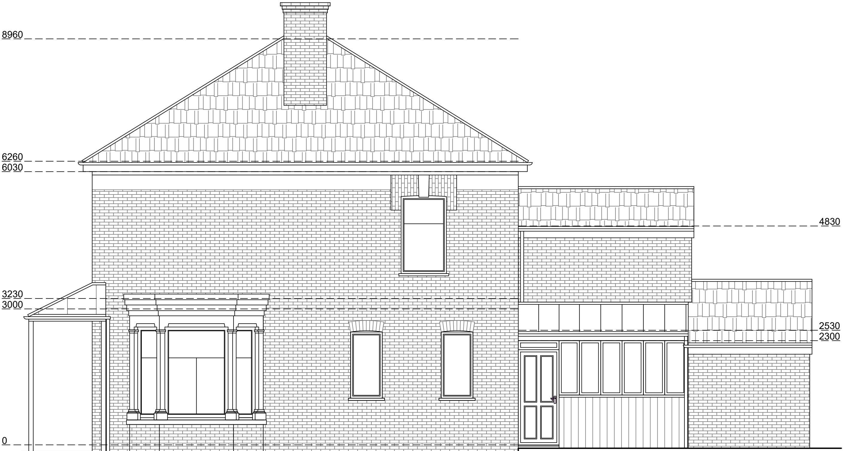
Existing North Elevation Scale 1:50
