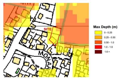
It can be seen that the area of the site where the house and the proposed extensions are located is within the "yellow" zone where the predicted flood depth is between zero and 250mm. The predicted hazard in this event is between zero and 0.75 (low hazard) for this area. Any proposed development would be categorised "F8" on the South East Lincolnshire Standing Advice Matrix. The standing advice for category "F8" is as follows for predicted flood depth of between zero and 250mm:
