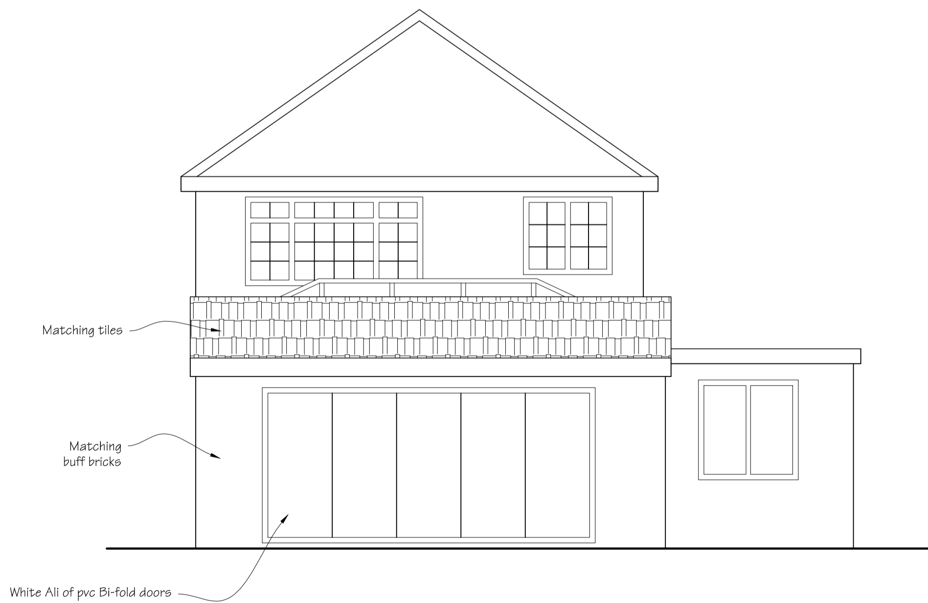
PROPOSED NORTH (Rear) ELEVATION Scale 1:50
